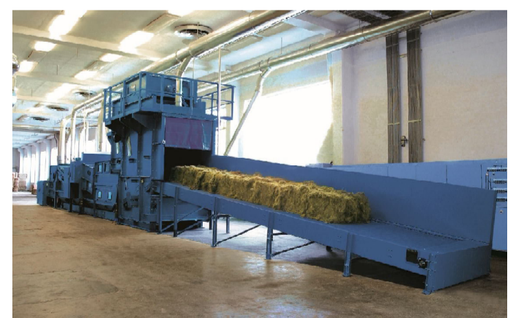
Fig. 2: Preparing the flax tow for the spinning mill on a Temafa machine
