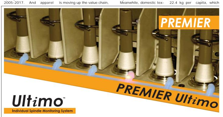
Ultimate Monitoring Solution for Ring Spinning Machines to optimise Energy, Man Power, Productivity and Quality with Individual sensor for each Spindle: updates LIVE information on Production, Yarn Break Data, Yarn Piecing Time, Machine Idle, Doff Duration, Rogue Positions, Efficiency, Kwhr per kg, Slip Spindles and Exceptions.
