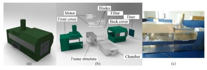
Fig. 3 -(a) Three-dimensional model of Kapok fibre seeds separator. (b) Exploded view of the 3-D model. (c) The prototype of product without finishing look (.https://www.researchgate.net/publication/342850134 Mechanical Design and Evaluation of Kapok Fibre Seeds Separator)
