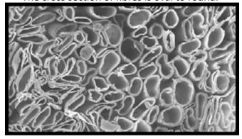
Fig. 5: Microscopic structure of kapok fibre, Microphotograph taken with a Scanning Electron Microscope — Transverse cross-sectional view of kapok fibres.
