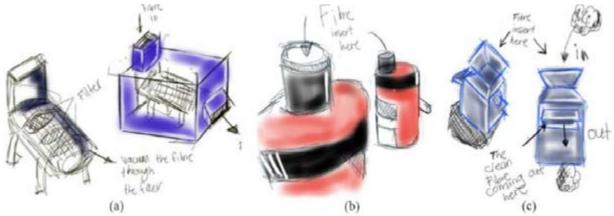
Fig. 2 -Three different design concepts of Kapok fibre seeds separator, (a) concept A, (b) concept B, and (c) concept C.
