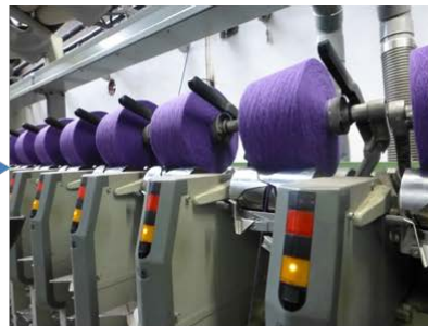
Open-end spinning => recycled yarn
