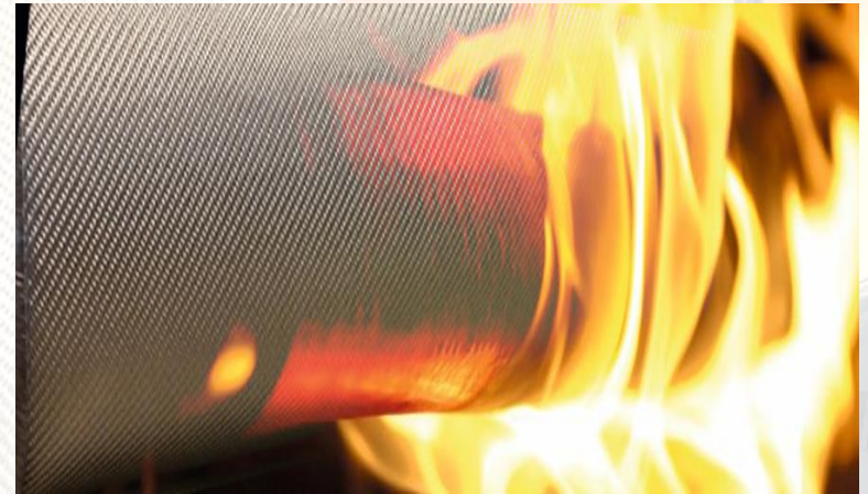
Thermal insulations for continuous operating temperature in range of 850 to 1.000°C
