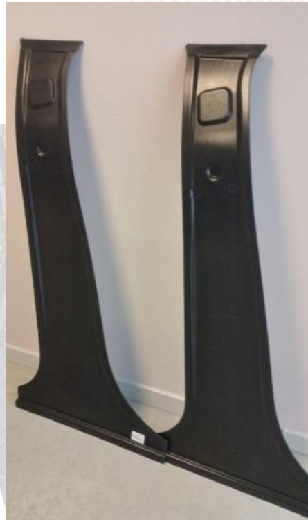
B-pillars and most critical structural supports
