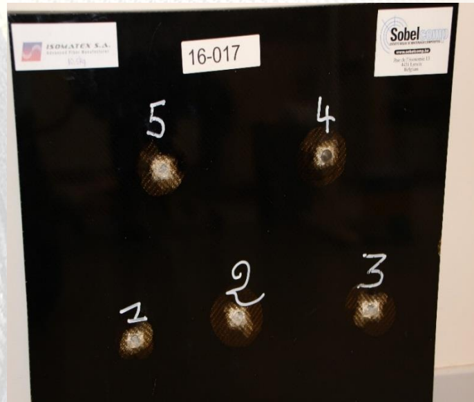
Bullet proof armour panel: the whole fibre reinforcement
