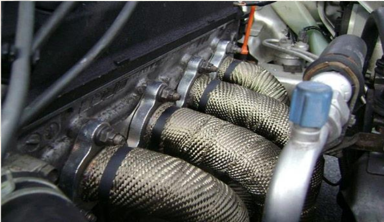
High-Temperature knitted or braided Sleeves for exhaust pipe protection
