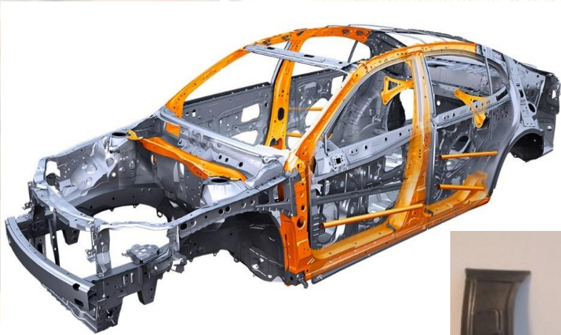
B-pillars and most critical structural supports
