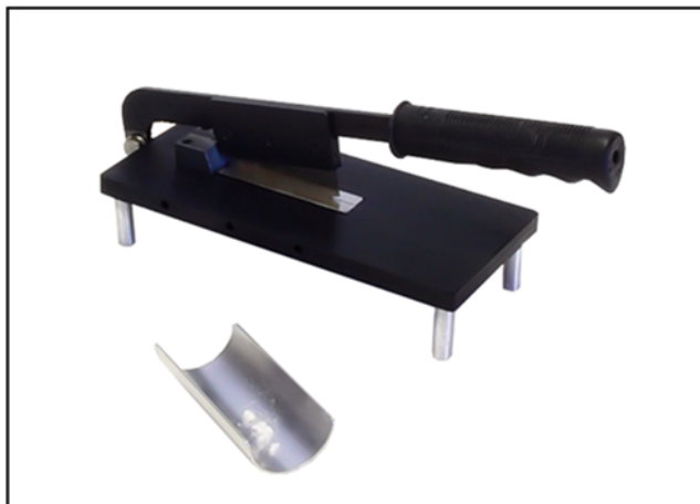
Fig. 5 Picture of benchtop guillotine used to prepare fibre snippets for evaluation
