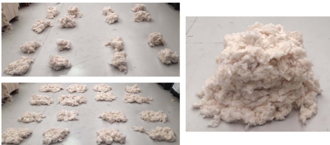
Figure 42: (left) The 16 subsamples after the 3 rd subdivision from the sample of step 4; (right) the sample at the end of the third mixing procedure, ready to be used in testing.
