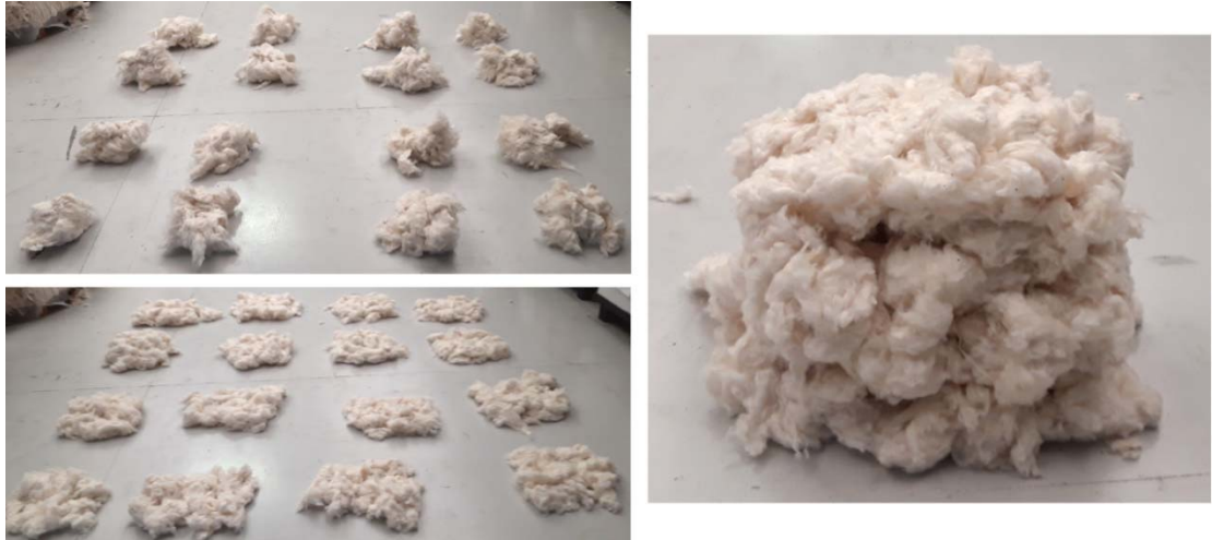
Figure 41: (left) The 16 subsamples after the 2 nd subdivision from the sample of step 3; (right) the sample at the end of the second mixing procedure.
