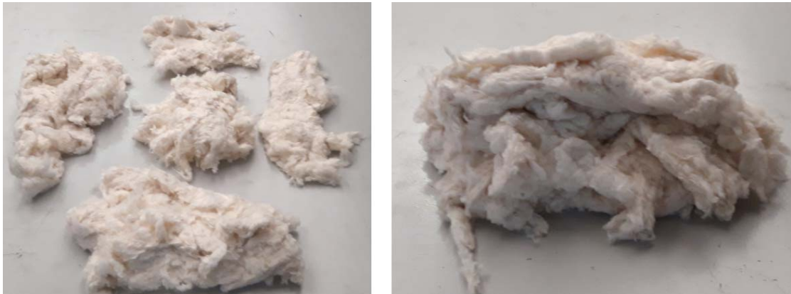
Figure 35: Step 1: (left) different portions taken from a single bale, (right) overlapping of the portions to create the starting sample.
