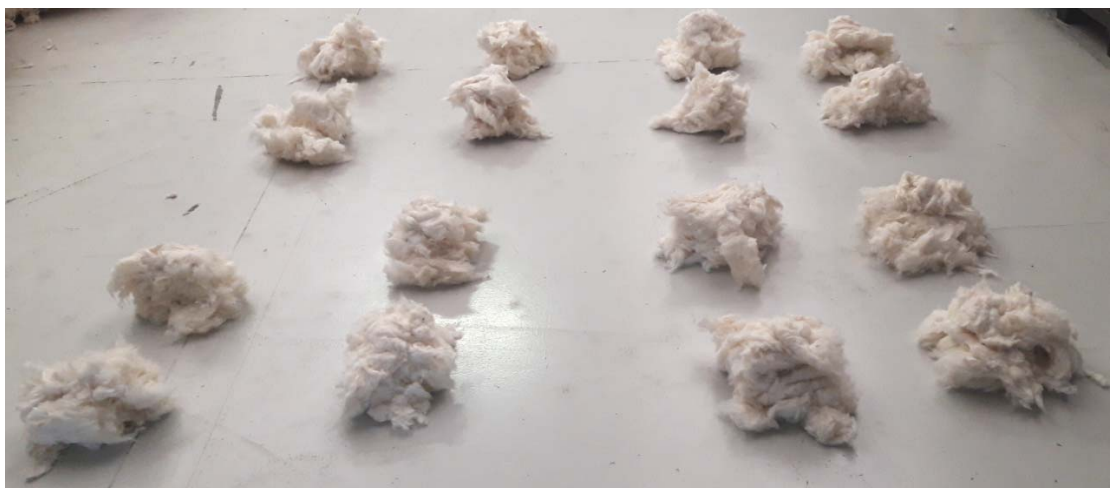
Figure 36: The 16 subsamples after the 1 st subdivision from the starting sample (step 2).
