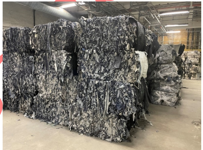
Photo 2: Cotton-rich textile waste as feedstock for new viscose fibres
