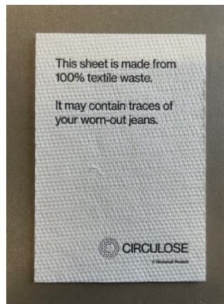
Photo 4: Final product "Circulose"; a sheet of pulp cellulose used for cellulosic fibers
