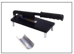
Fig. 4 Picture of benchtop guillotine used to prepare fibre snippets for evaluation
