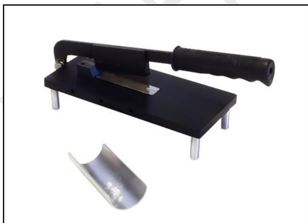
Fig. 5 Picture of benchtop guillotine used to prepare fibre snippets for evaluation
