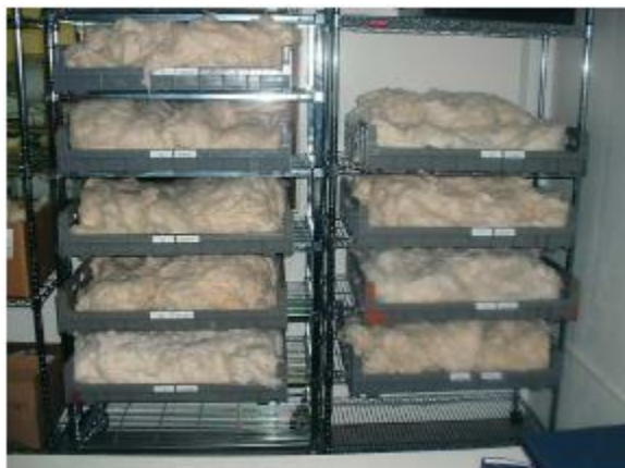
Figures: Storage of samples for conditioning [Uster]
