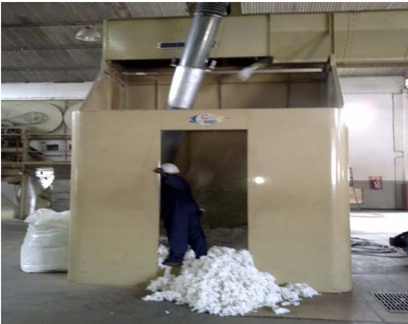
Plexus gins the seed-cotton with saw-gins at low speed which preserves the good properties of the fibre.
